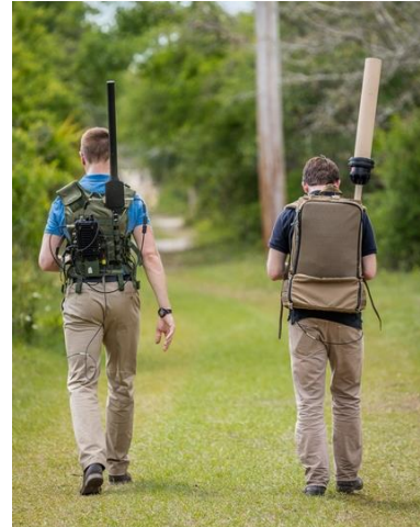
Sabre Antenna (left) vs. JTWS GSK stock Antenna (right)
